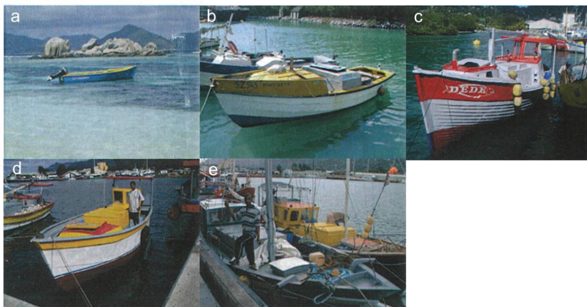
Figure 1 Artisanal fishing vessels within the Seychelles: (a) Mini Mahe; (b) Lekonomi; (c) Whaler; (d) Lavenir; and (e) Schooner.
